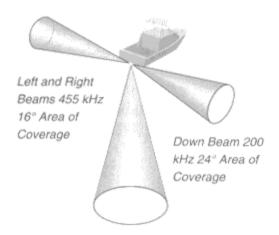
The Wide Side transducer is available as a trolling motor mount, a transom mount, or a portable mount.
